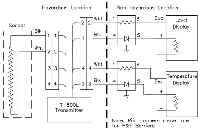
Figure 2.12 Wiring to level/temperature displays with excitation
