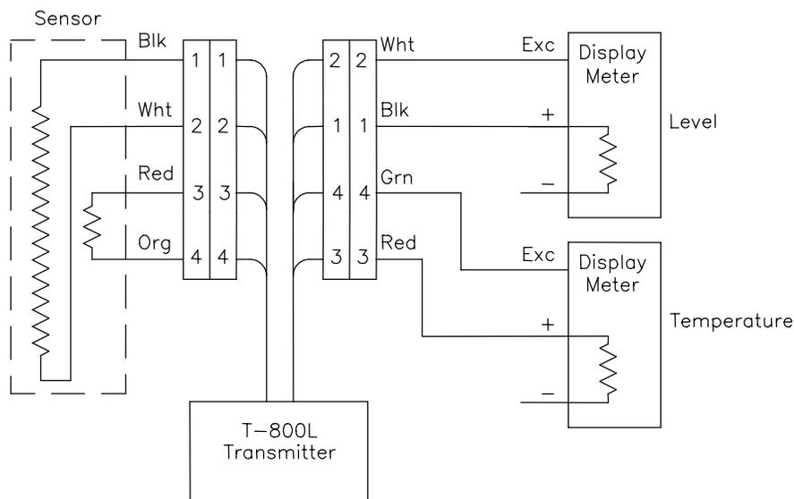
Figure 2.7 Level/temperature wiring to display with excitation
