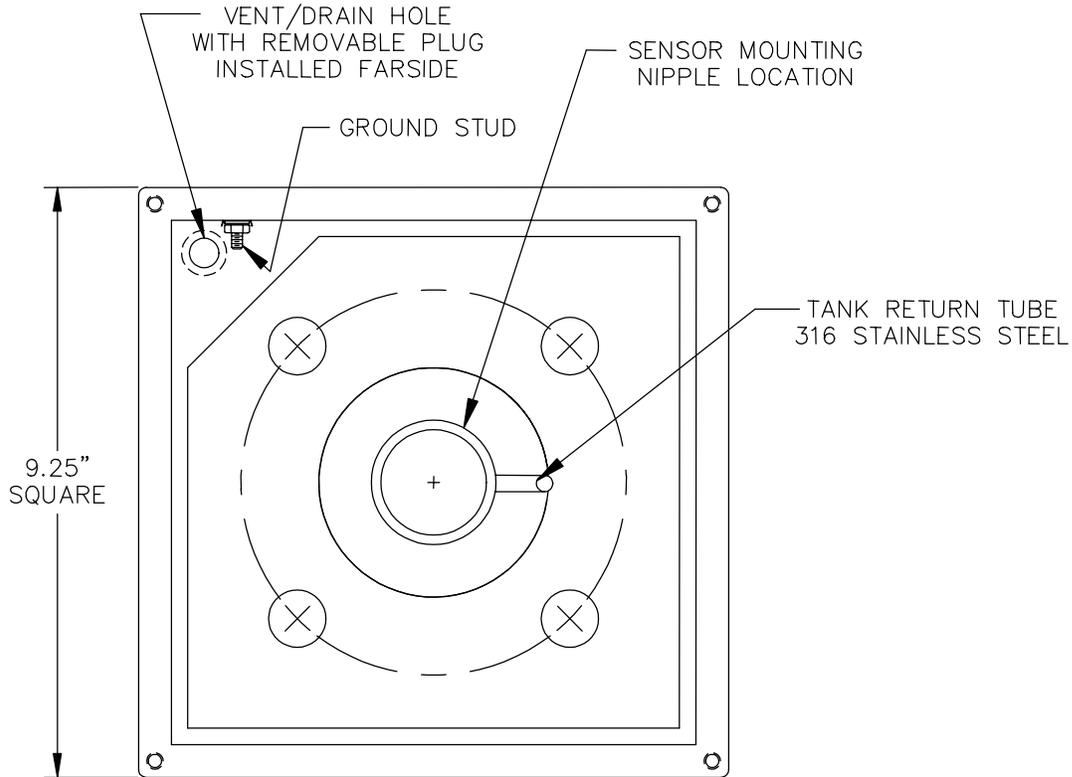
Figure 1.4 Sensor Housing – Top view with cover removed
