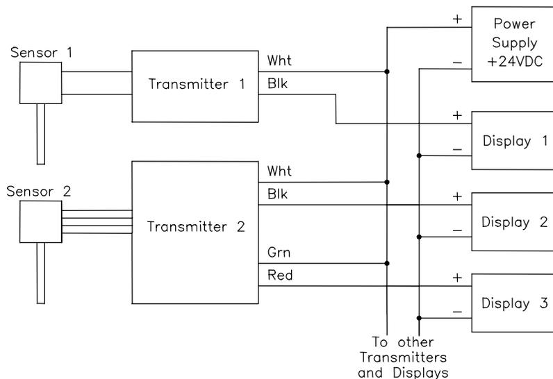
Figure 2.3 Powering multiple transmitter channels
