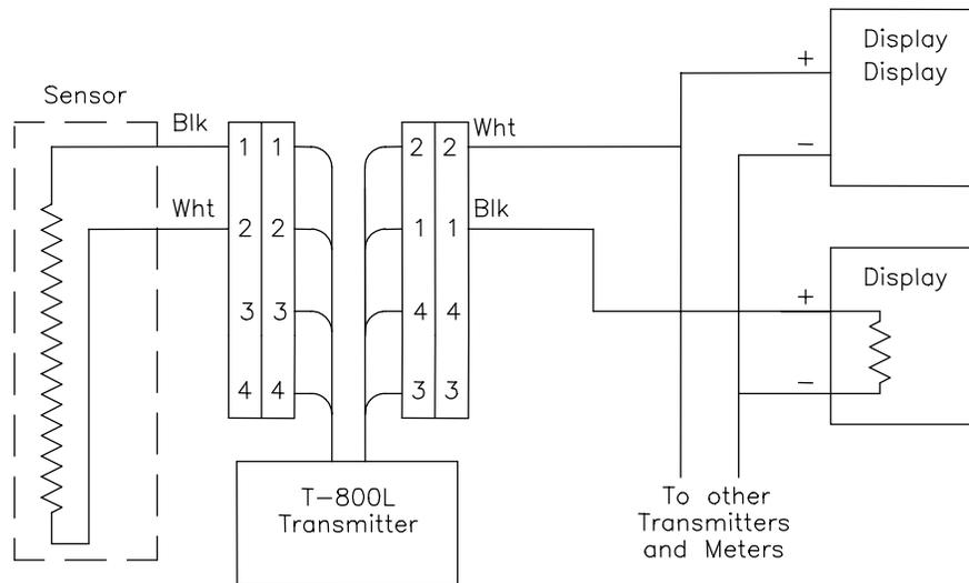
Figure 2.6 Wiring to display with separate power supply
