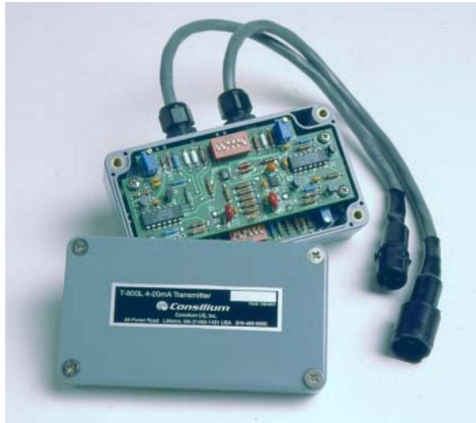
Figure 1.5 Current Transmitter
