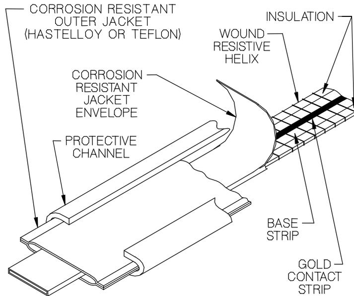
Figure 1.2 Cutaway view of the Petrotape/Chemtape Sensor
