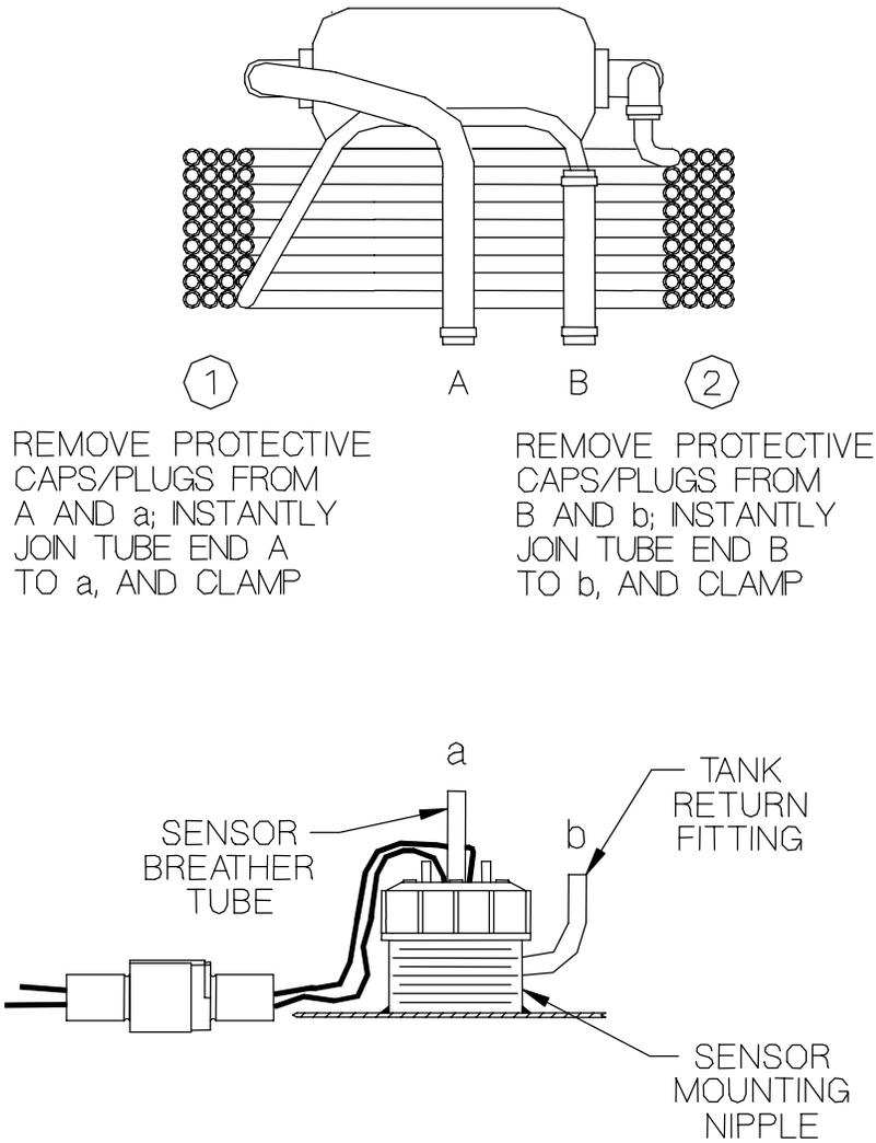
Figure 3.3 Connecting the filter to the sensor
