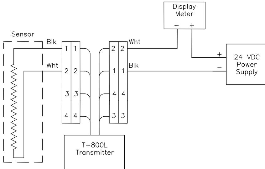
Figure 2.4 Level Wiring to Process Current Display
