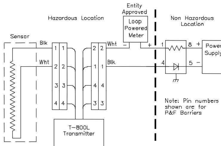
Figure 2.9 Hazardous location wiring to entity approved loop powered meter
