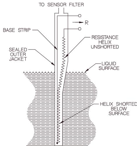
Figure 1 Sensor Operation
