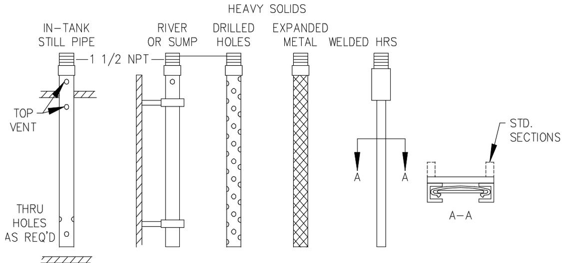
Figure 3 Sensor mounting for various liquid viscosities
